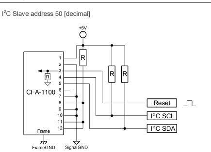
Connect the frameGND with the frame, otherwise with the F.G. through-hole.
