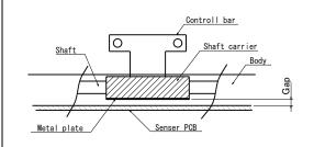
Simple structure of a sensor board and the metal plate which do not touch it each other.
